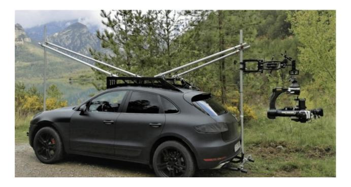
The Flowcine Black arm is a 3-axis suspension system with a vibration mount for stabilizing roll and tilt axes as well as vertical movements and vibrations. The Black Arm is a hardmount system, made for remoteheads, that you can use on vehicles such as cars, ATVs, boats, snowmobiles, etc. With the Flowcine Black Arm it is easy to reduce the effects of shocks, vibrations and bumps during filming with a camera on a vehicle, dolly or other moving platform.
