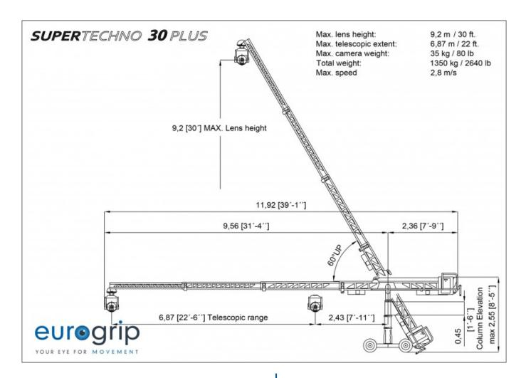
With the Supertechno 30 plus you can perform complex camera movements without necessarily moving the dolly. The Supertechno 30 plus has a telescopic reach of 6.87m and a height range of 9.20m. All our Techno 30's are equipped with a speed box, which almost doubles the speed of the extendable arm. The Supertechno 30 comes with a Z-Head as standard but can also be used with other heads.
