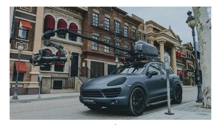
The U-Crane Dynamic is a new generation of our gyrostabilized robotic camera crane systems. It is a remotely operated gyrostabilized minicrane technology that was designed for use on small camera cars, electric carts, process trailers or other small tracking vehicles to be able perform on narrow roads, small sized sets, tunnels, parking garages, bridges.
