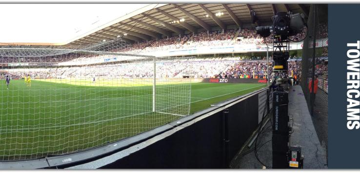
The MAT–Tower-Cam is a remote-controlled, telescopic column, which can be combined with a remote head (360 ° pan). The column moves smoothly and precisely and is almost completely silent. The maximum lens height for this model is 4.6 meter.
