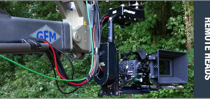
This head that hangs by default under the Super Technocranes, can support almost every camera (both video and film) and is fully modular. It can be built with 2 or 3 axes, in different sizes.
